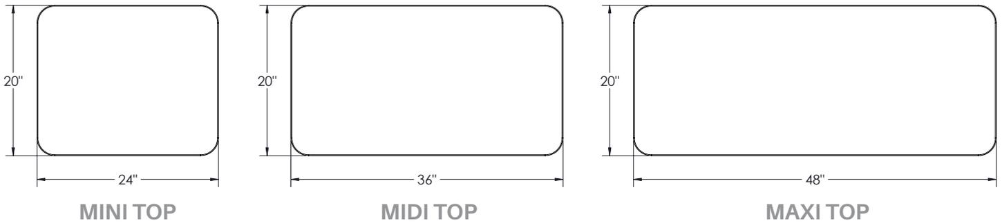
\*\*Laminate tops are 1 1/8" thick particle board core with HPL and 3mm T-mold Edge\*\*
